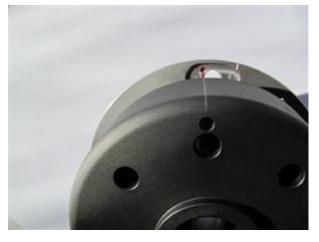
With the piston in ignition position replace the rotor carefully on the crankshaft, aligning the timing marks on the adapter plate and the circumference on the rotor (see left). Screw it down with the original mounting nut.
