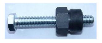
To disangage the new rotor again, you need a puller M27x1,25 (part 99 99 799 00 -Not provided!-).
