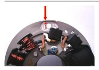
Put the preassembled stator unit onto the engine case, like the original was installed. Fasten it with the 3 screws M6x20 centrically at the oblong holes.
