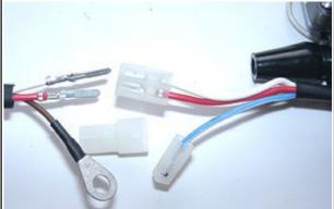
Look for the ignition coil with its female plug and the two wires (red and white).
